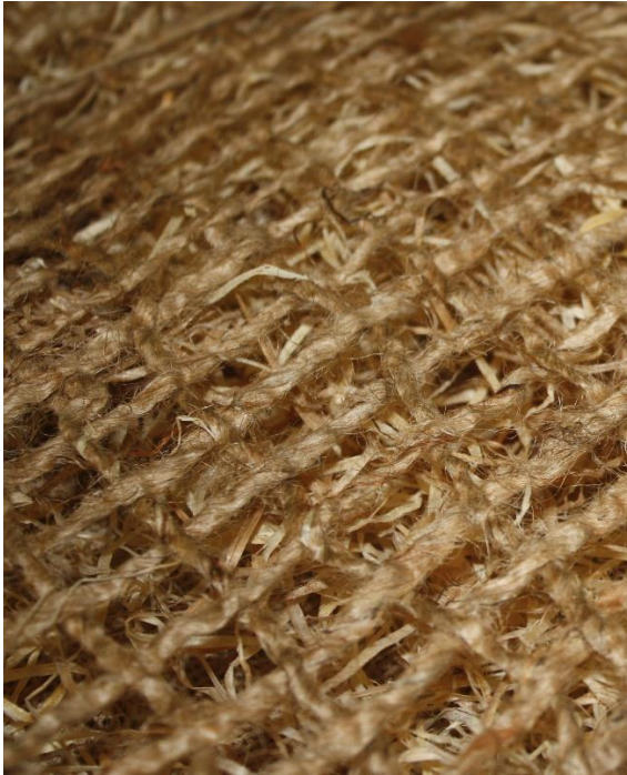
Figure 5.12 Narrow view of Sedimat with layered jute mesh and wood wool
