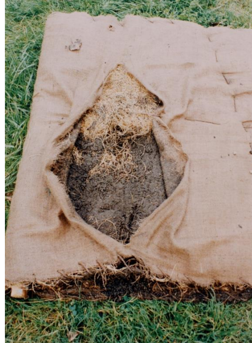
Figure 5.13 “Full” Sedimat after having been removed from stream bed
